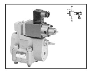
This current-controlled type relief valve has been developed for continuous and stepless remote control of hydraulic circuit pressure. To control the pressure, the current input to the DC solenoid in the pilot section is controlled by the control amplifier, thus directly controlling the poppet action with the attraction force of the solenoid.
