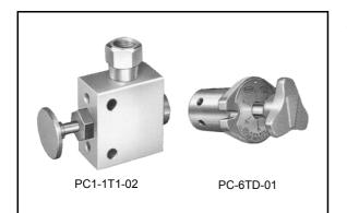
The pressure checker is used to allow through or shut off the hydraulic fluid flow to the pressure gauge. When the pressure checker is used, one pressure gauge can check the pressure for up to six circuits. In addition, since pressure is applied to the pressure gauge only during measurement, the pressure gauge can be protected from damage and its life prolonged.
