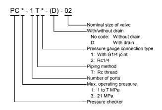
**NOTE:** The PC1 series is "without drain" and the PC3 series is "with drain".
